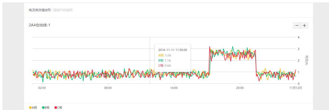
High Voltage Side Abnormal Current of the Load Transformer
